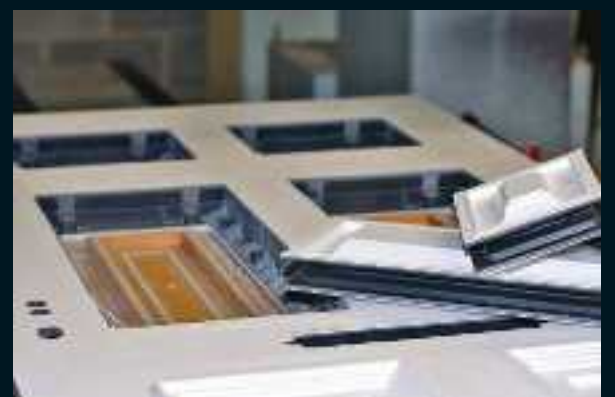
Door after routing operation
