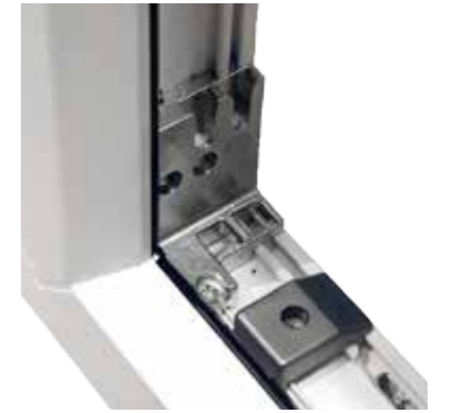
High security multipoint shootbolt lock. When activated, shootbolts engage firmly into keeps fitted to the window frame to add extra security.
